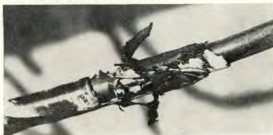
Some typical lightning damage. The F-100 was struck more than 100 times during Rough Rider '64.
