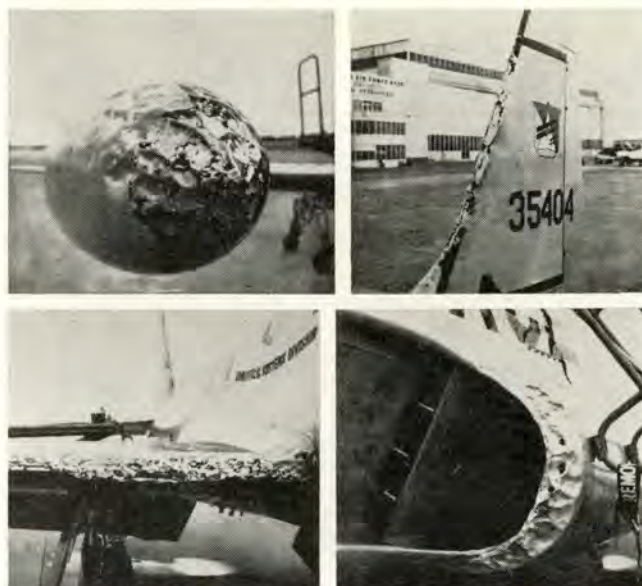
During Rough Rider '62, a T-33 penetrated a mild-looking thunderstorm. Note hail damage. Author says appearance no criteria.
