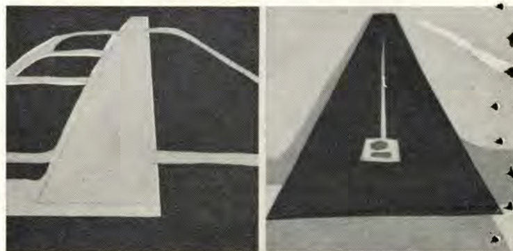
How long is the runway? A narrow, short runway can appear to be the same size as a long, wide runway. Don't guess. Check approach plates.
