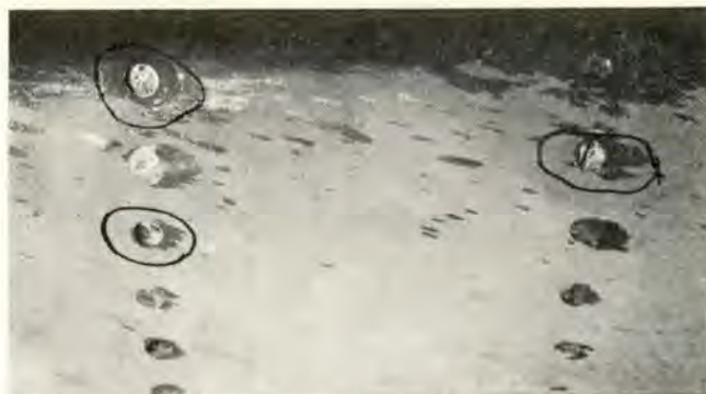
F-106 wing leading edge flush rivets that were peeled by rain impingement during supersonic penetrations of severe thunderstorms.
